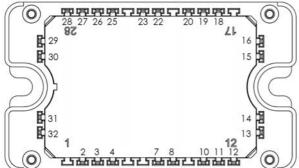
Pins 29/30/31/32 must be shorted together Pins 26/27/28/22/23/25 must be shorted together to achieve a phase leg Pins 16/18/19/20 must be shorted together  $V_{CES} = 1200V$  $I_{C} = 180A$  @  $T_{C} = 100$ °C
