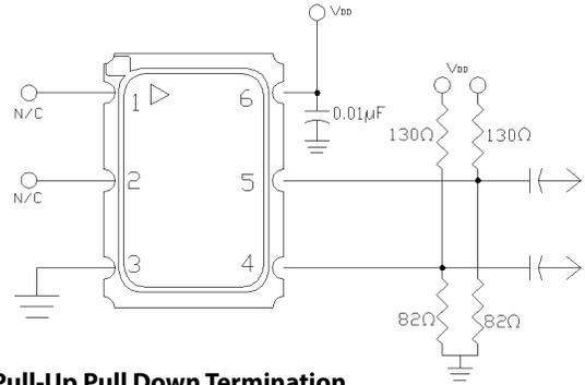
**Figure 12. Pull-Up Pull Down Termination**
