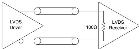
**Figure 13. LVDS to LVDS Connection, Internal 100ohm Resistor**
