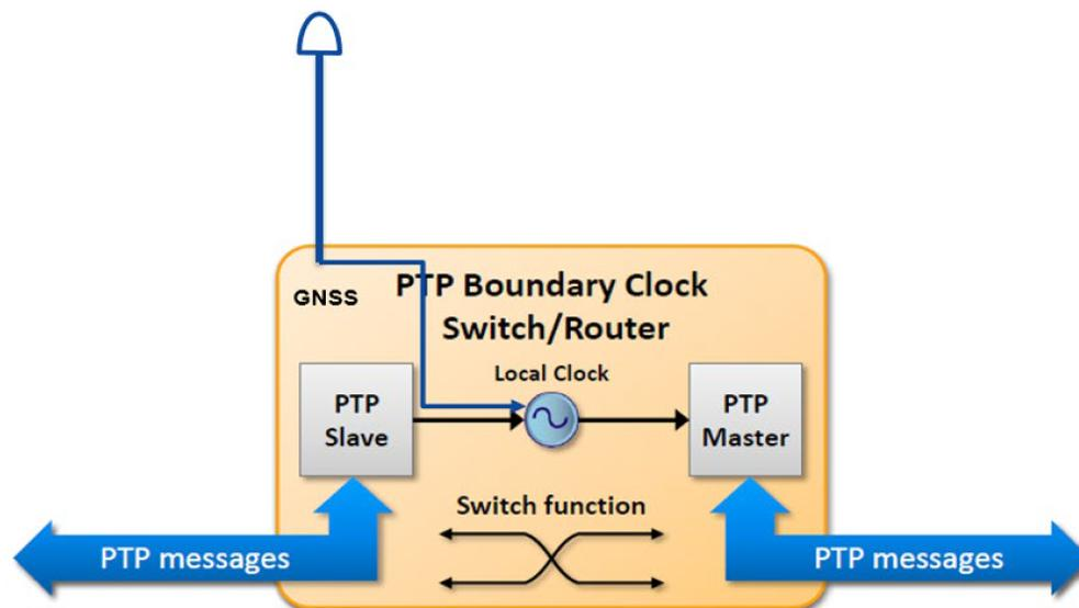
The timing functions can operate in two modes; first, as a GMC by adding a local GNSS antenna to the system; and second, when deployed without the GNSS, as a G.8273 Boundary Clock (BC) receiving PTP packets from a GMC deployed upstream in the network.
