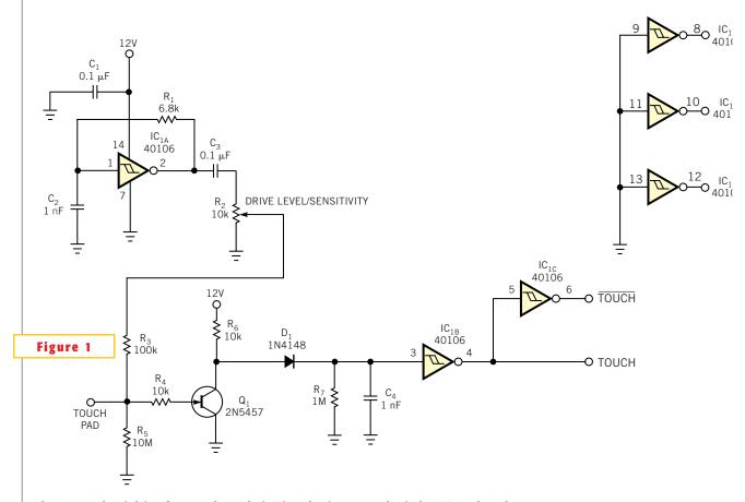
A low-cost touch-switch interface uses three Schmitt trigger hex inverters and a single JFET per channel.
