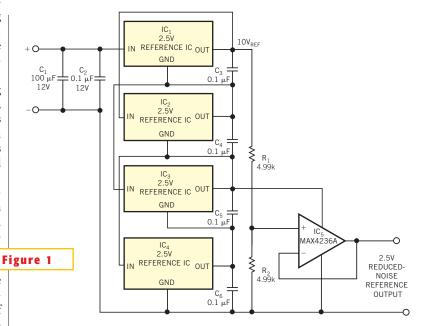
Four 2.5V references,  $IC_1$  through  $IC_4$  produce 10V. Resistors  $R_1$  and  $R_2$  form a voltage divider that reduces the 10V output to 2.5V and lowers the output-noise voltage by half. Buffer amplifier  $IC_5$  isolates the reference circuit from the load.
