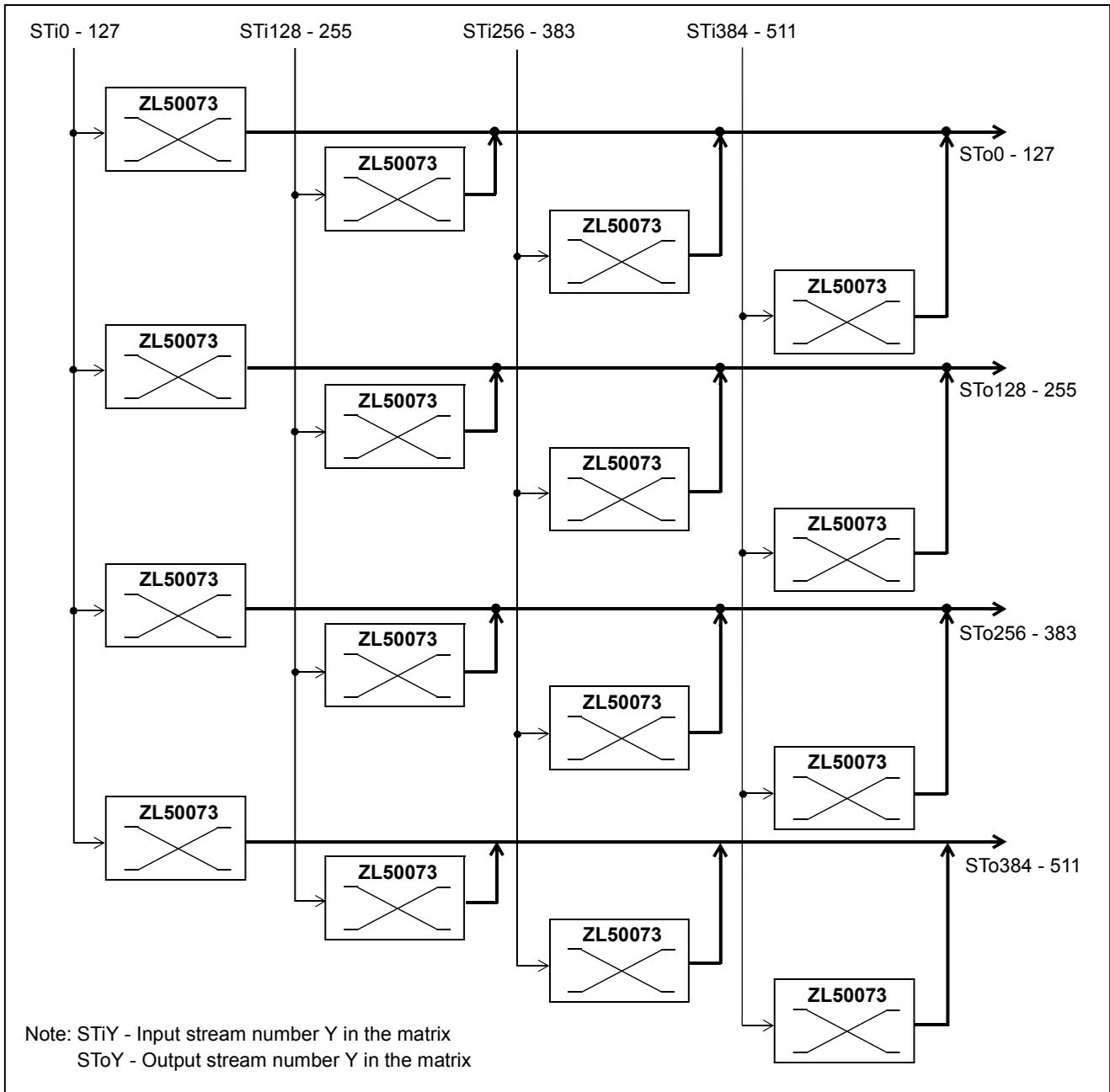
Figure 3 - 128 K x 128 K Non-Blocking Square Switching Matrix
