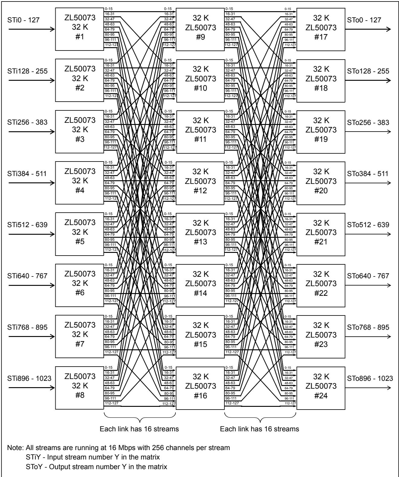
Figure 5 - 256 K x 256 K Three-Stage Matrix
