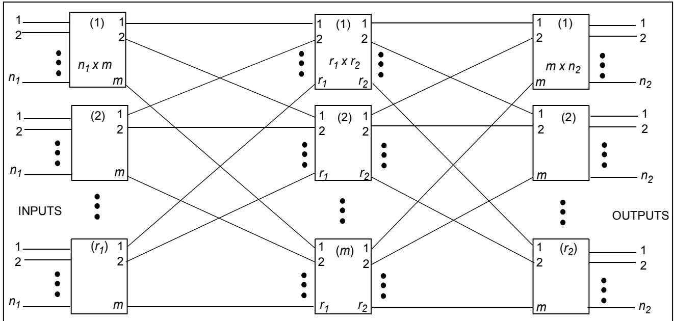
**Figure 4 - General Structure of a Three-Stage Switching Matrix**
