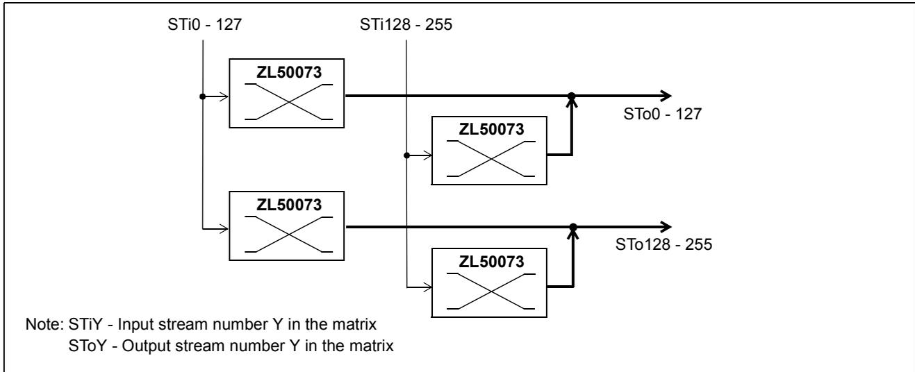
**Figure 2 - 64 K x 64 K Non-Blocking Square Switching Matrix**
