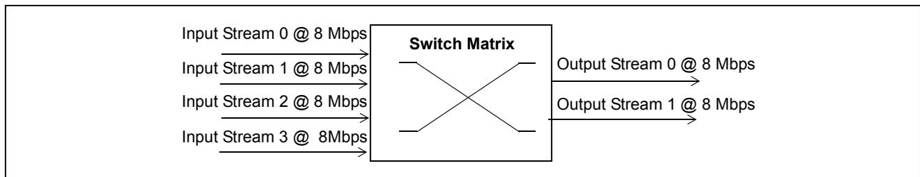
Figure 1 - Blocking Switch Matrix
