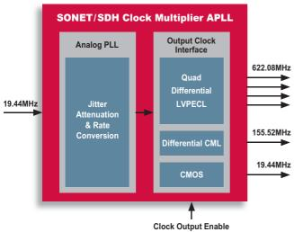
The ZL™ 30414 is the world's first SONET (synchronous optical network) and SDH (synchronous digital hierarchy) clock multiplier analog phase locked loop (APLL) to provide six output clocks from a single device with jitter performance that surpasses OC-192 and STM-64 system requirements. This unique level of integration and performance allows designers of SONET and SDH networking equipment to meet stringent timing requirements.
