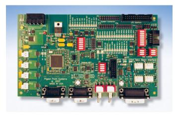
A complete hardware and firmware solution for the mandatory Enhanced Module Management Controller (EMMC) on MicroTCA modules such as OEM modules or cooling units. Kit includes:
