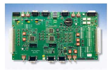
A complete hardware and firmware solution for the mandatory MicroTCA Carrier Management Controller (MCMC) on a MicroTCA Carrier Hub (MCH), which includes the MCMC, Carrier Manager, and an optionally installed Shelf Manager, all executing on a single microcontroller. Kit includes:
