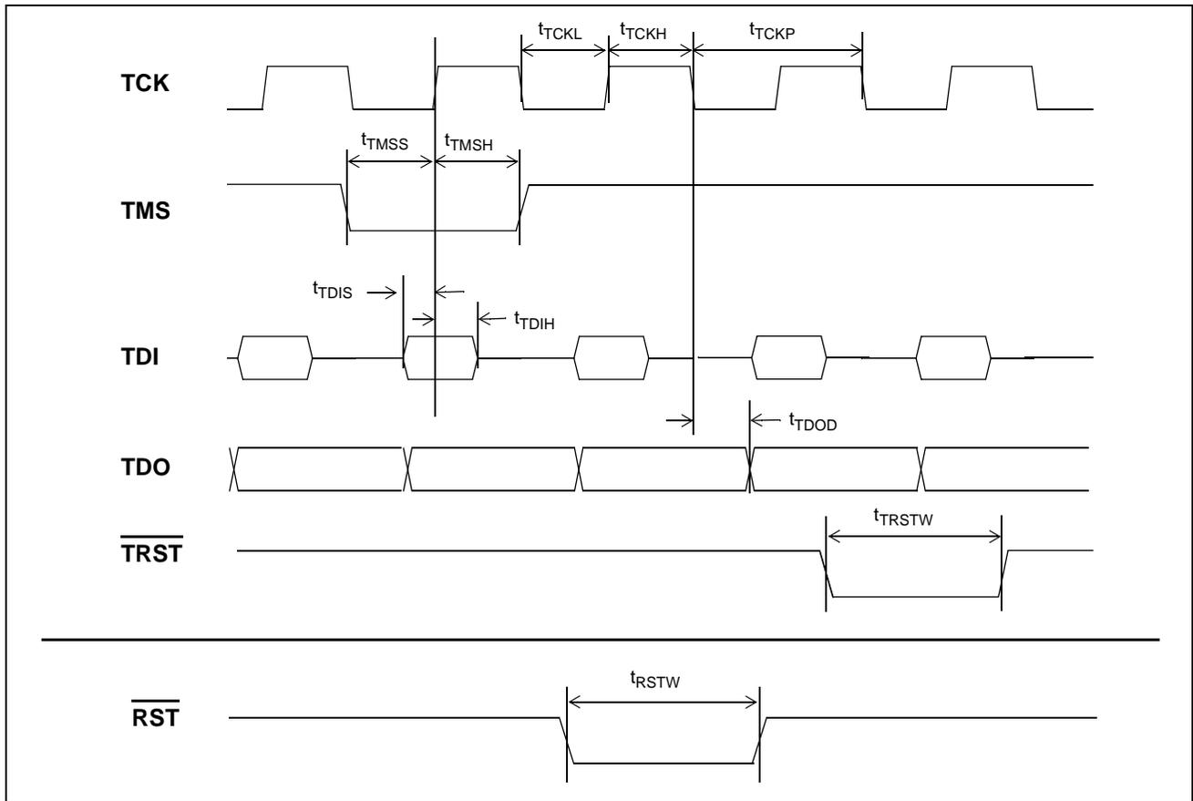
**Figure 54 - JTAG Test Port Timing**
