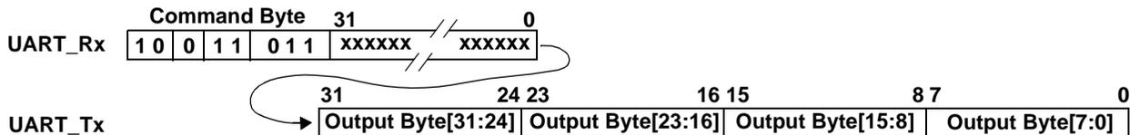
Figure 67 - UART Read Register Address 02A1<sub>H</sub>
