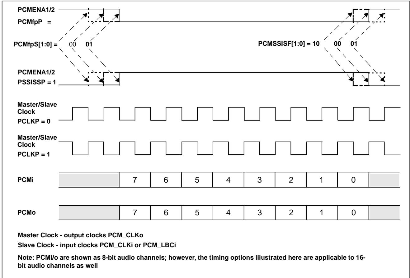
Figure 14 - SSI Slave/Master Enable and Bit Clock Functional Timing
