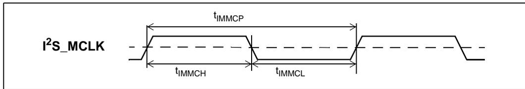
**Figure 50 - I<sup>2</sup>S Master Clock (MCLK) Timing**
