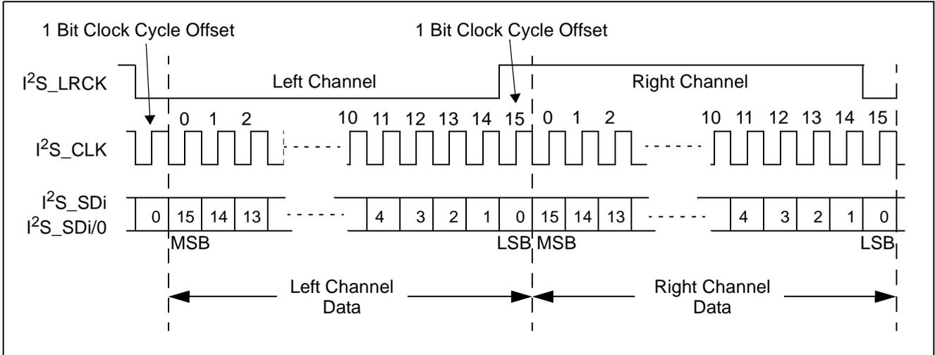
Figure 19 - I<sup>2</sup>S Audio Interface with Left Channel Enable Low/Right Channel Enable High
