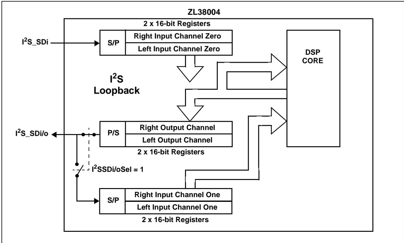
Figure 21 - Inter-IC Sound (I<sup>2</sup>S) Loopback
