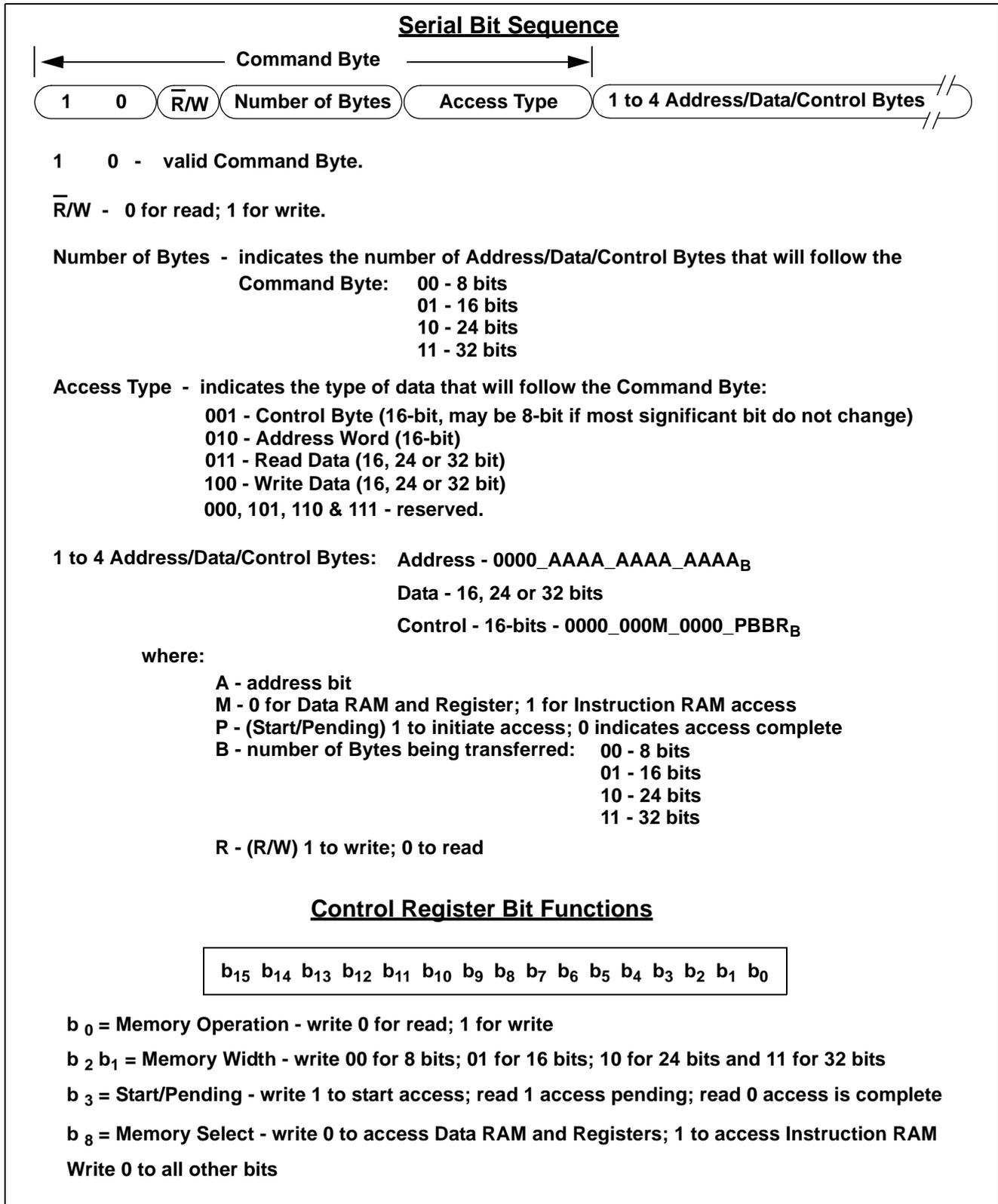
Figure 25 - Slave SPI and UART Port Access
