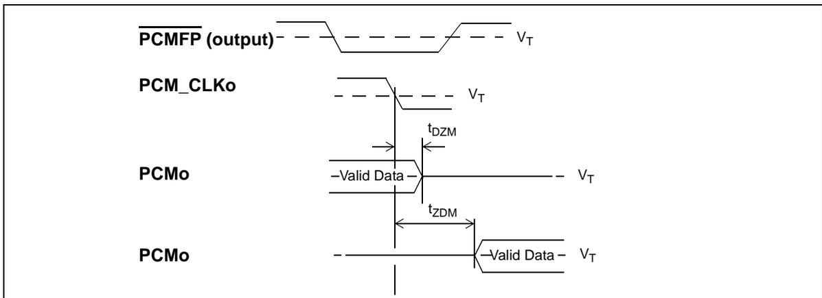
**Figure 42 - Output Tristate Timing in TDM Master Mode**
