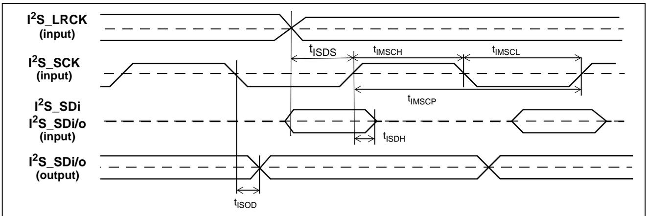
**Figure 49 - Slave I<sup>2</sup>S Timing**
