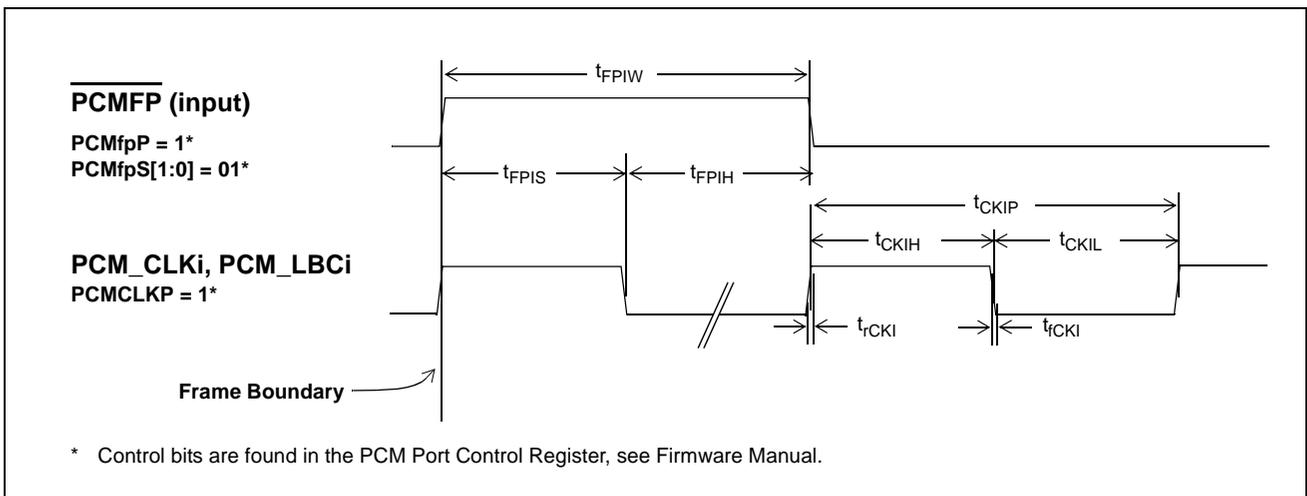
**Figure 37 - TDM - GCI PCMF $\overline{P}$  and PCM\_CLK $\overline{i}$ , PCM\_LBC $\overline{i}$  Input Timing**
