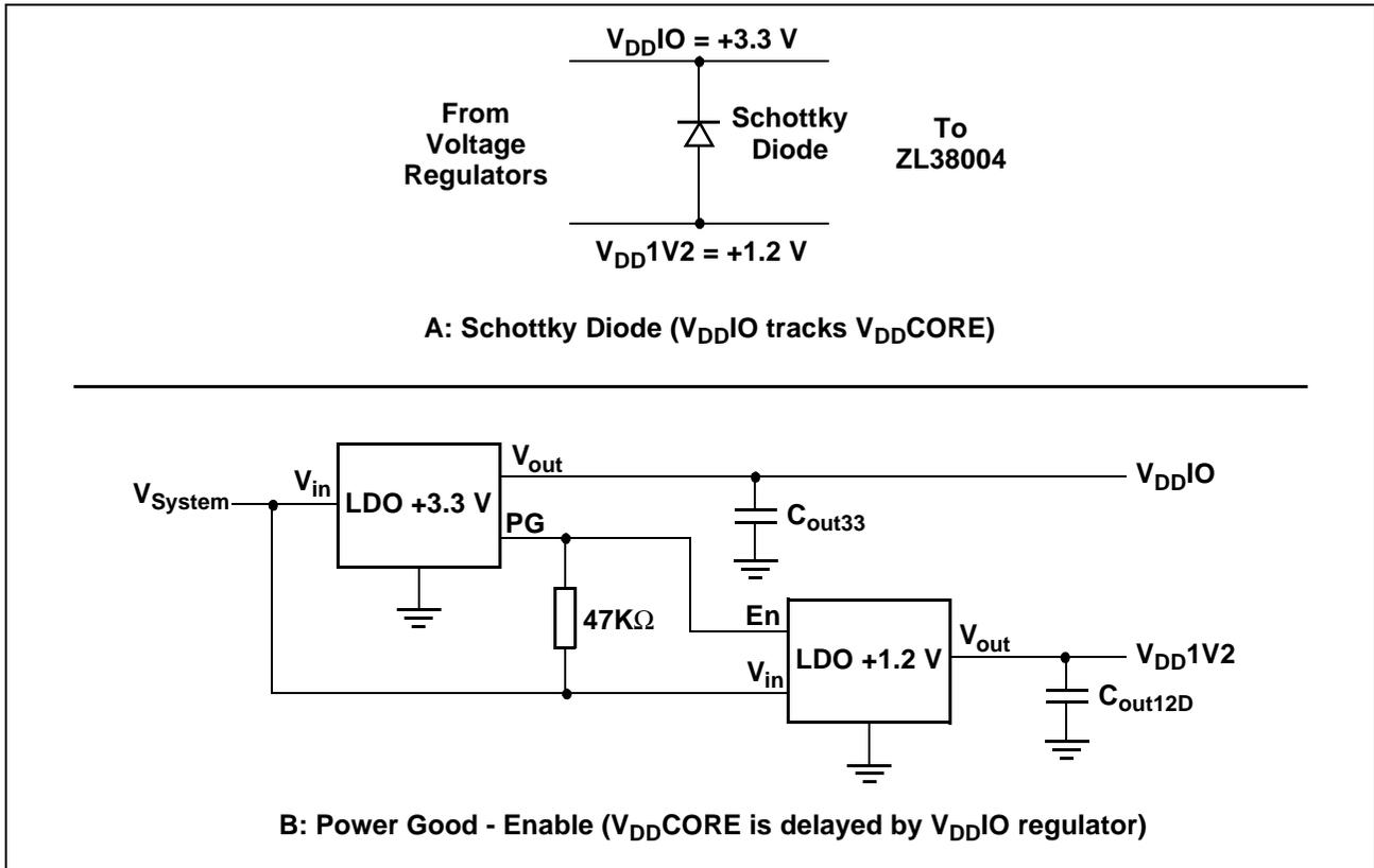
**Figure 55 - Latch-Up Prevention Circuit Options**
