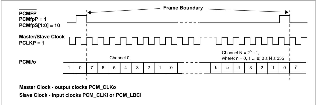
Figure 13 - TDM - McBSP Slave/Master Functional Timing Diagram
