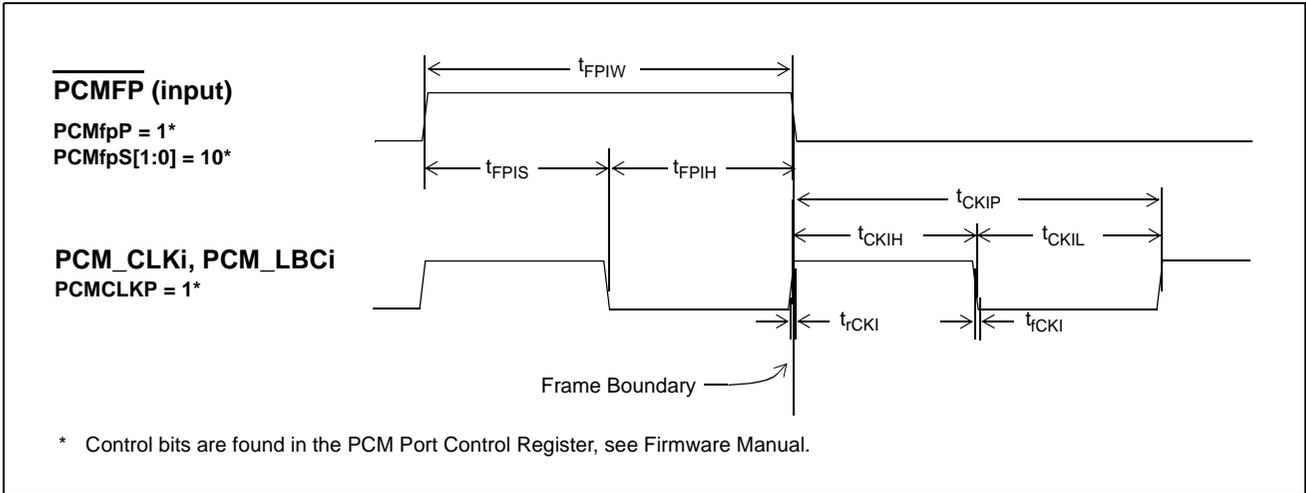
**Figure 38 - TDM - McBSP PCMFP and PCM\_CLKi, PCM\_LBCi Input Timing**
