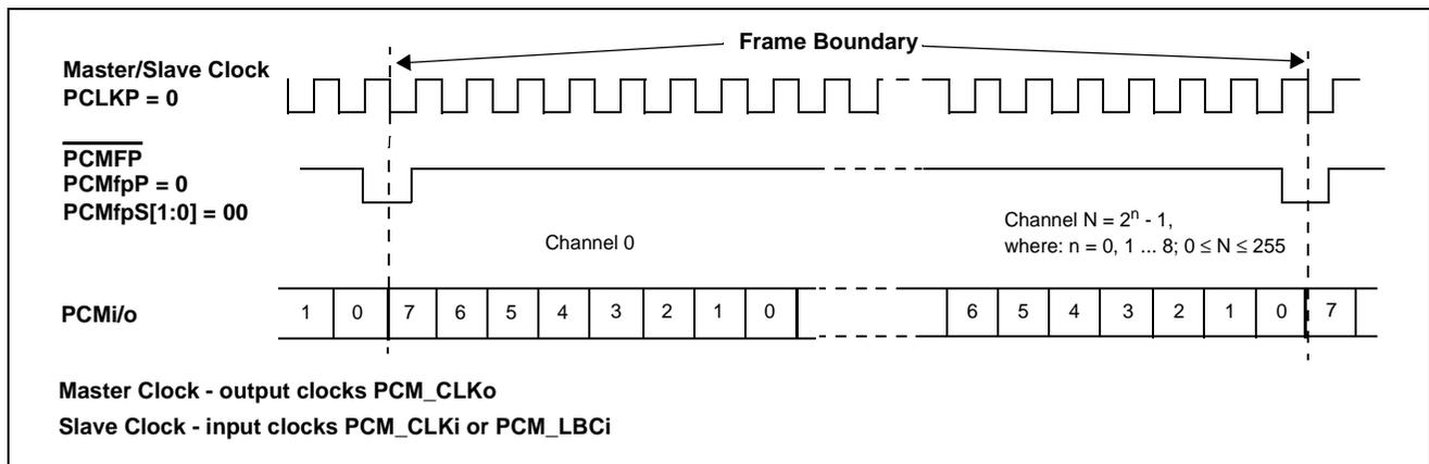
**Figure 10 - TDM - ST-BUS Slave/Master Functional Timing Diagram**
