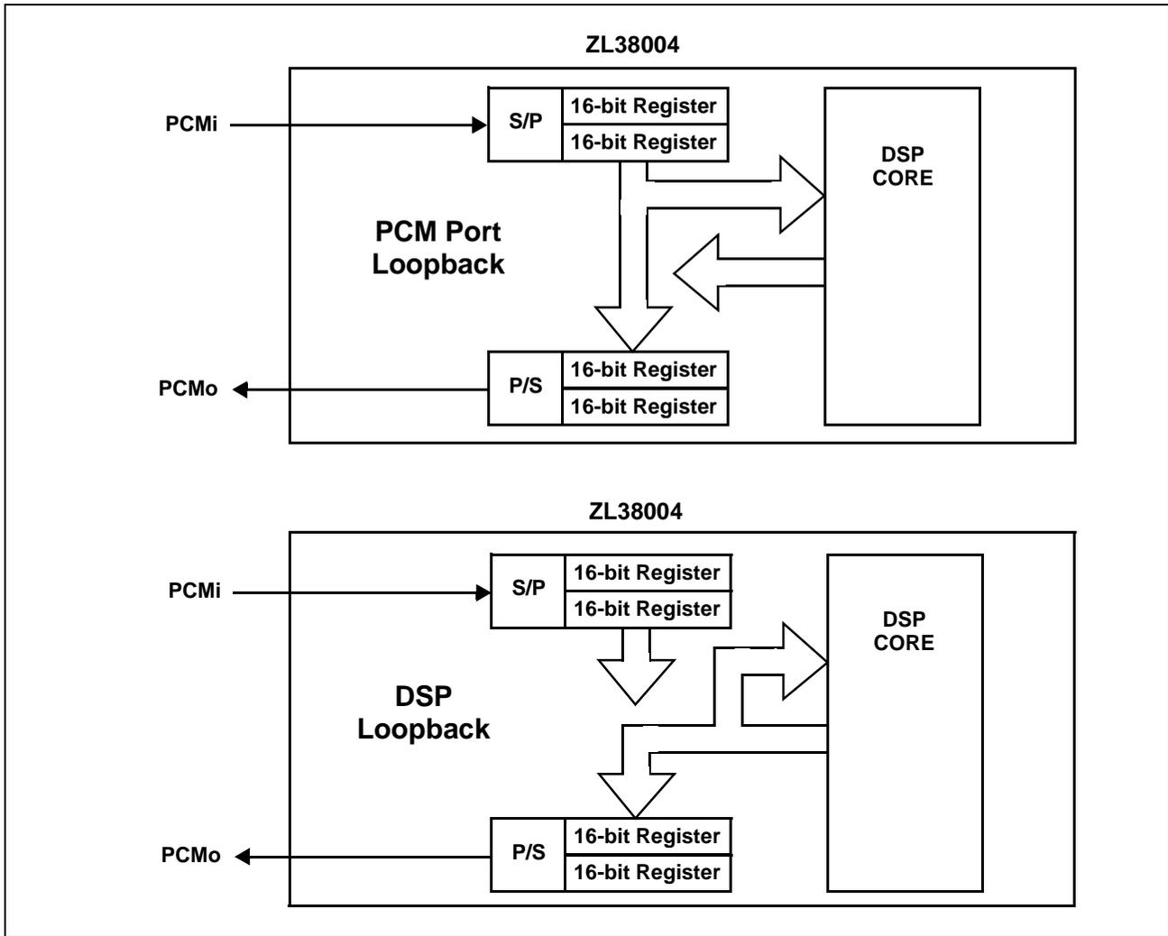
Figure 9 - PCM and DSP Loopbacks
