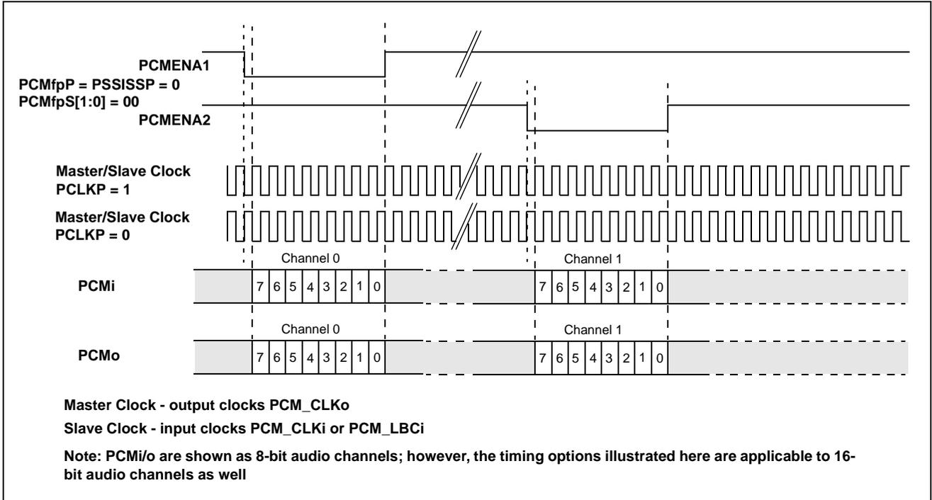
**Figure 15 - SSI Mode: Separated Channels Functional Timing**
