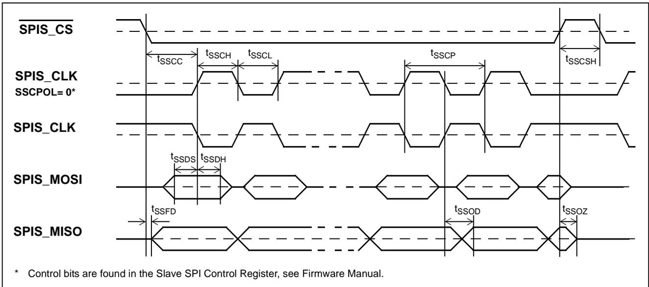
**Figure 44 - Slave SPI Timing (SSCPHA = 0)**
