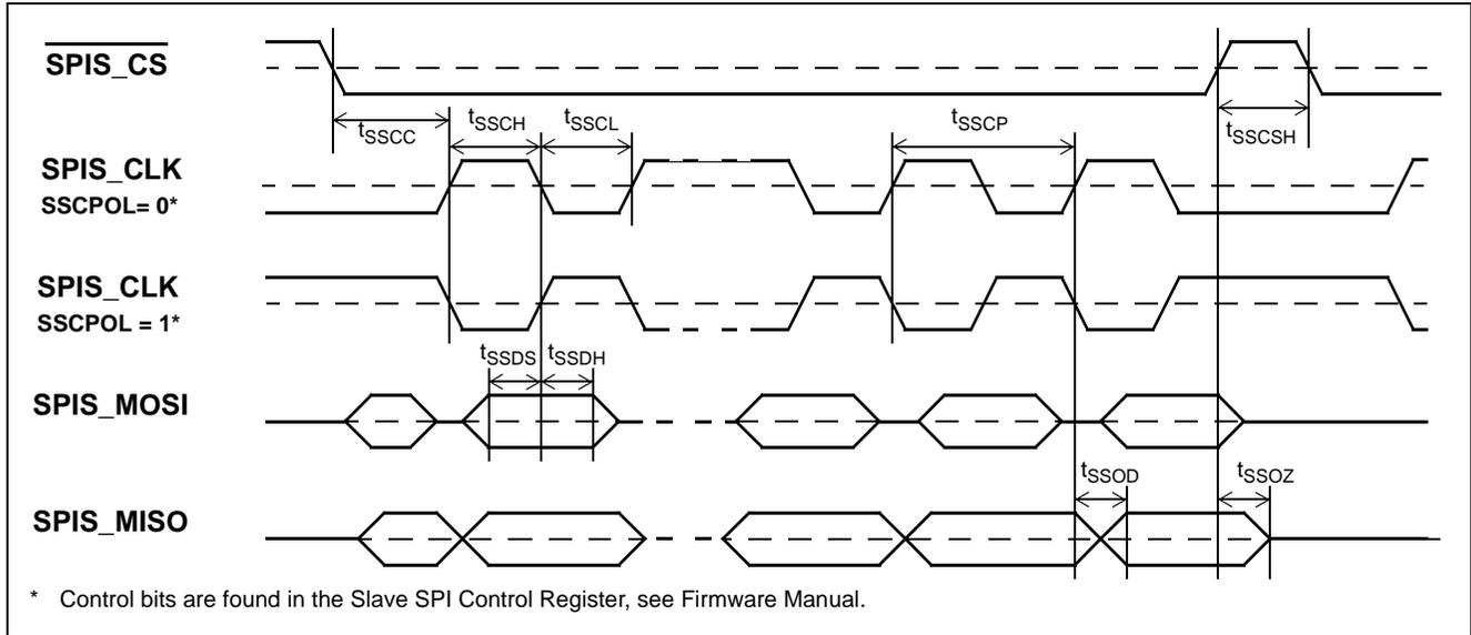
Figure 45 - Slave SPI Timing (SSCPHA = 1)
