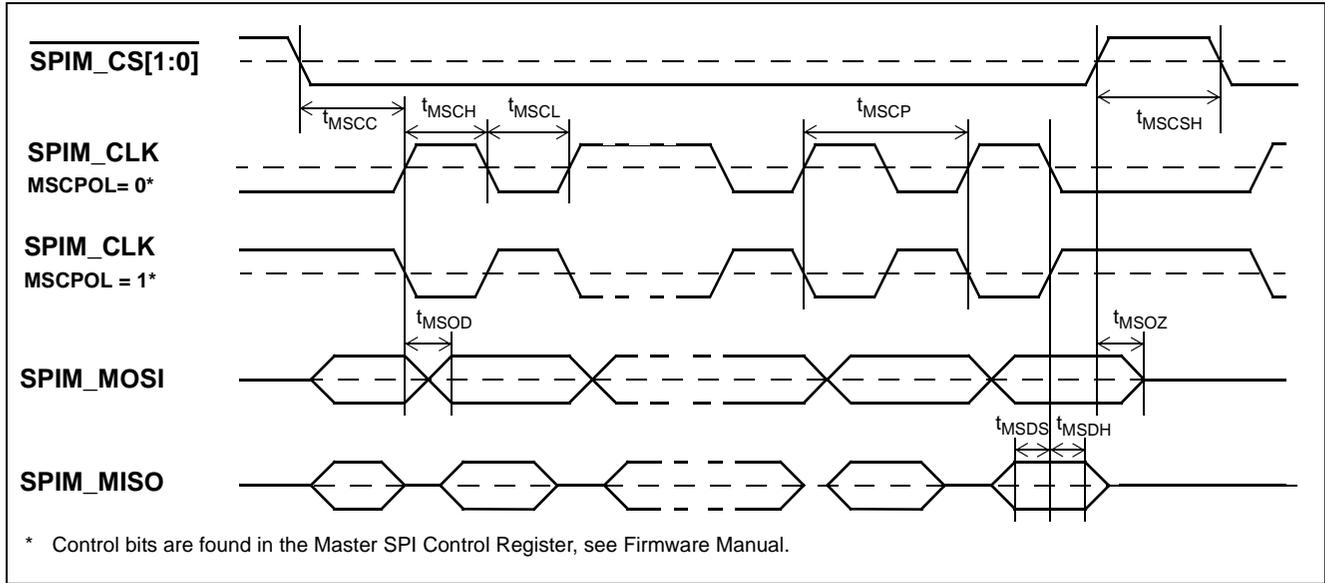
**Figure 48 - Master SPI Timing (MSPHA = 1)**
