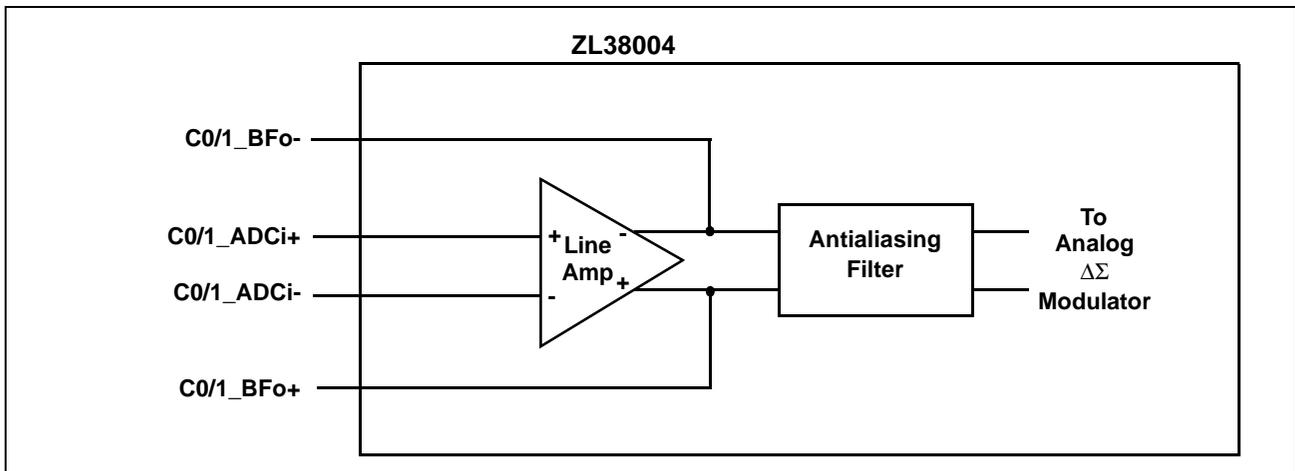
**Figure 5 - CODEC 0/1 ADC Line Amplifier Selected**
