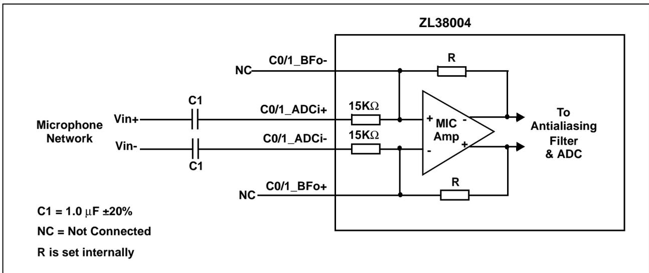
**Figure 59 - CODEC 0/1 ADC Differential Microphone Amplifier Circuit**
