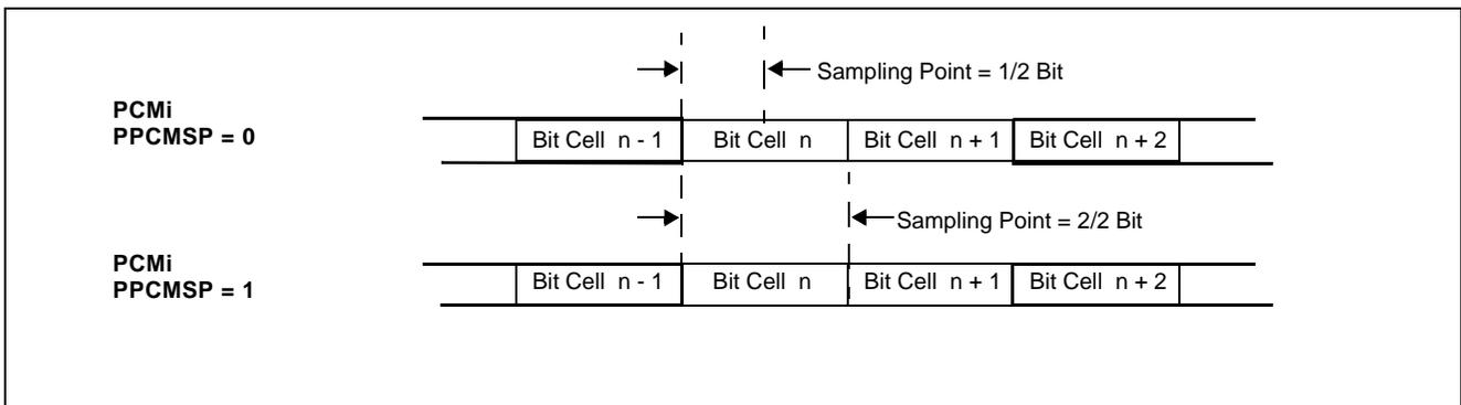
**Figure 8 - PCM Serial Data Input Sampling Points**
