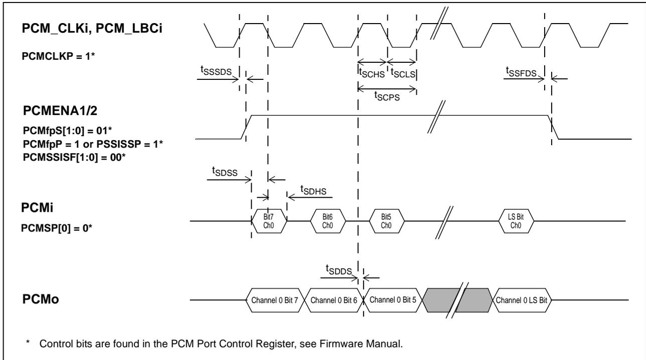
**Figure 34 - PCM SSI Slave Mode Timing Diagram**
