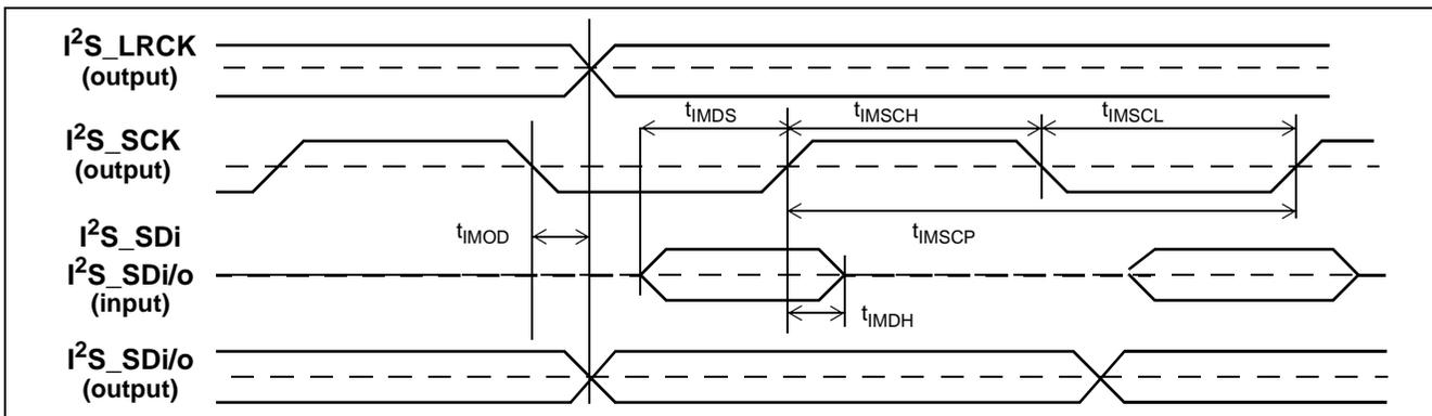
**Figure 51 - Master I<sup>2</sup>S Timing**
