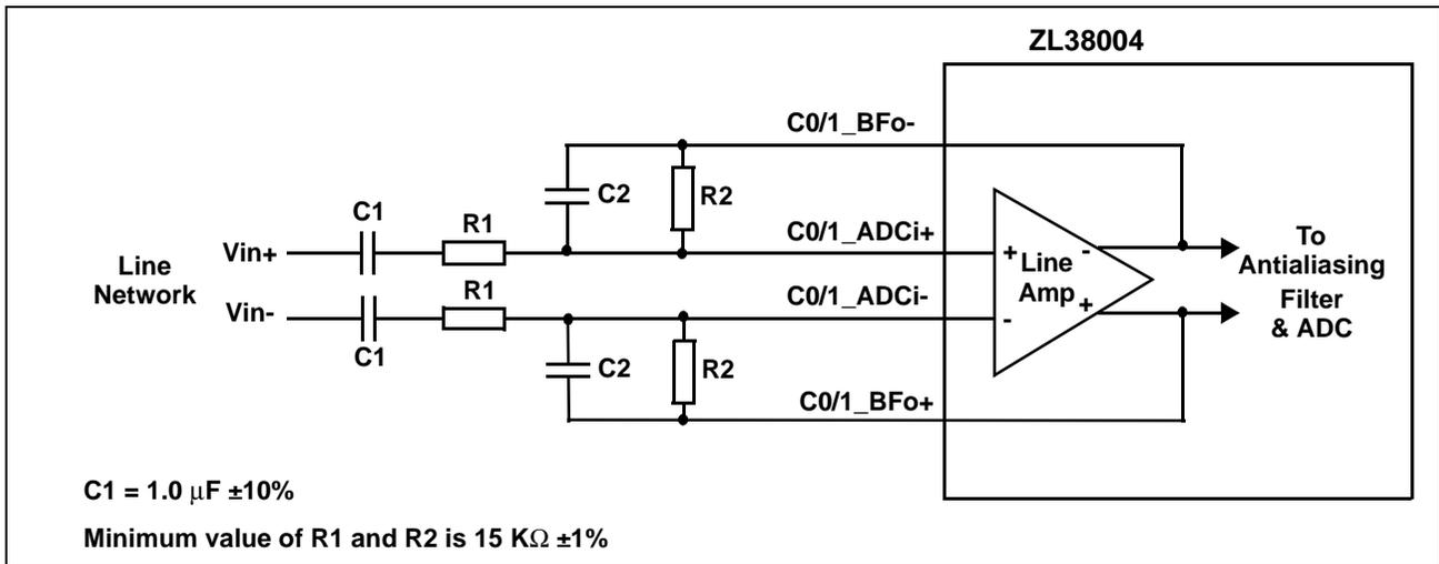
Figure 60 - CODEC 0/1 ADC Differential Line Amplifier Circuit
