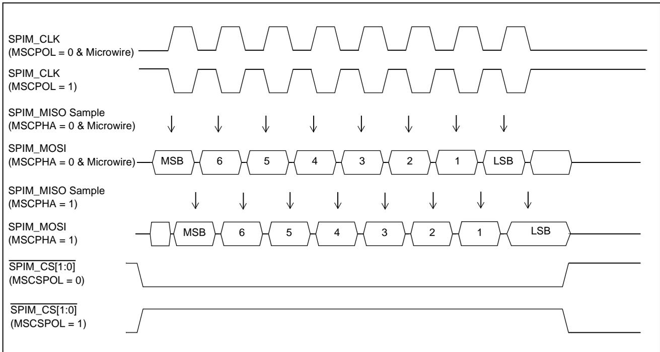
**Figure 22 - Master SPI and Microwire Port Functional Timing**
