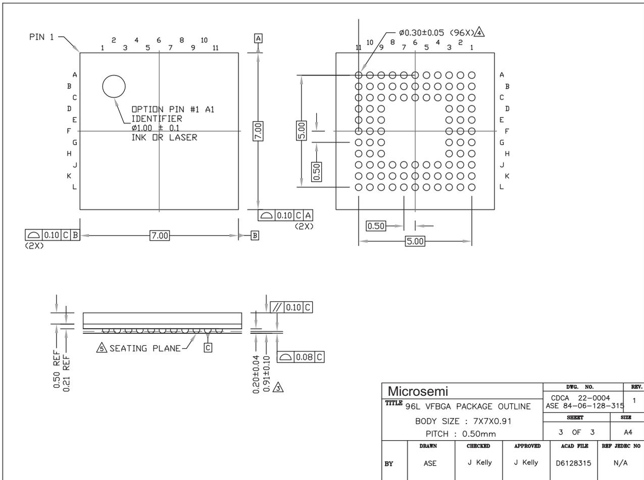
**Figure 70 - ZL38004 (96-Pin CABGA) Package Drawing**
