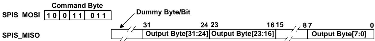
Figure 65 - SSPI Read Register Address 02A1<sub>H</sub>
