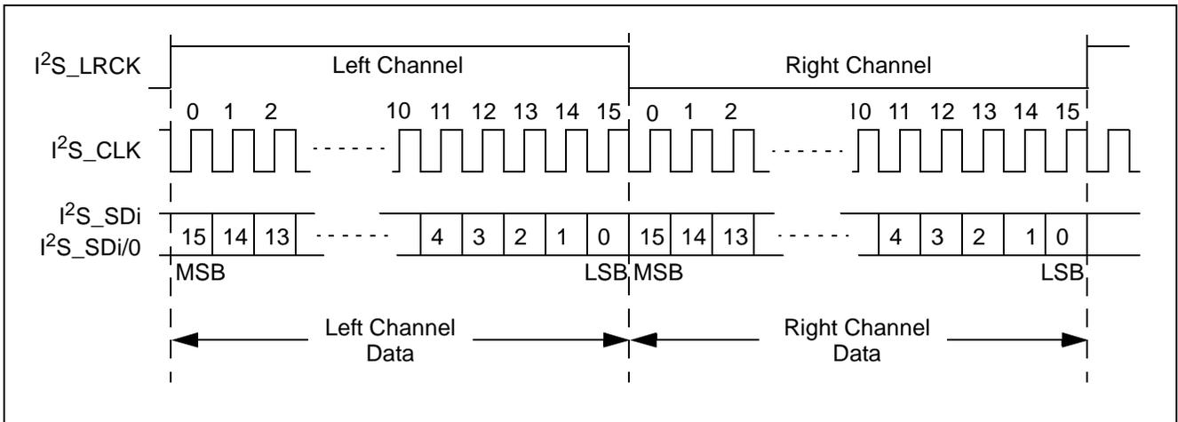
Figure 20 - I<sup>2</sup>S Audio Interface with Left Channel Enable High/Right Channel Enable Low
