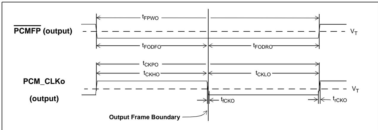
**Figure 43 -  $\overline{\text{PCMFP}}$  and PCM\_CLKo TDM Master Mode Timing**
