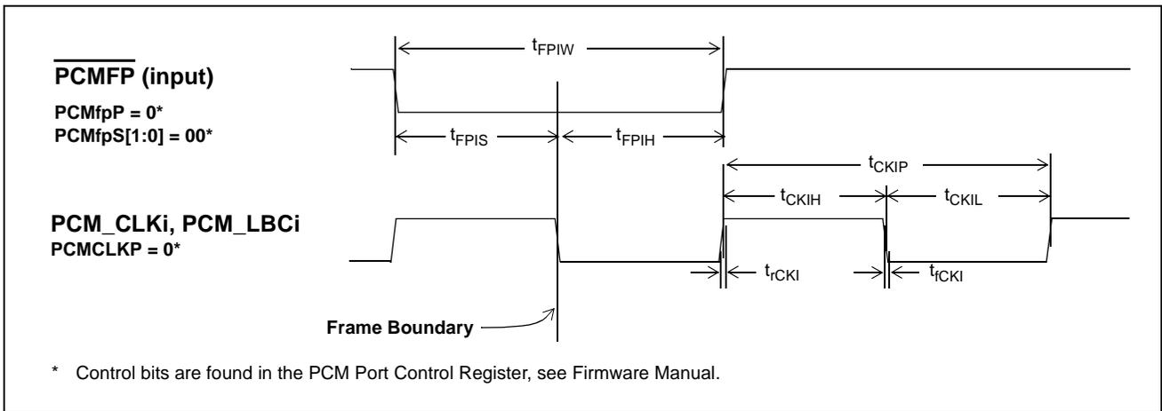
**Figure 36 - TDM - ST-BUS PCMF $\overline{P}$  and PCM\_CLK $\overline{i}$ , PCM\_LBC $\overline{i}$  Input Timing**
