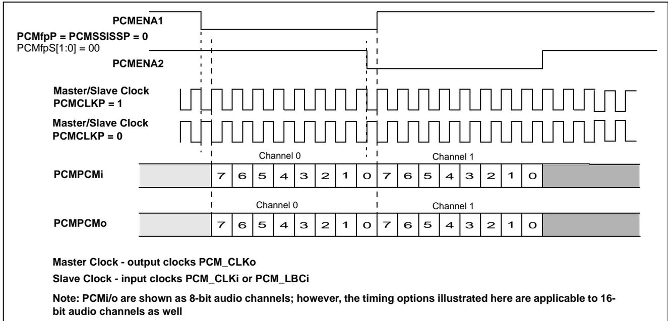
Figure 16 - SSI Mode: Adjacent Channels Functional Timing
