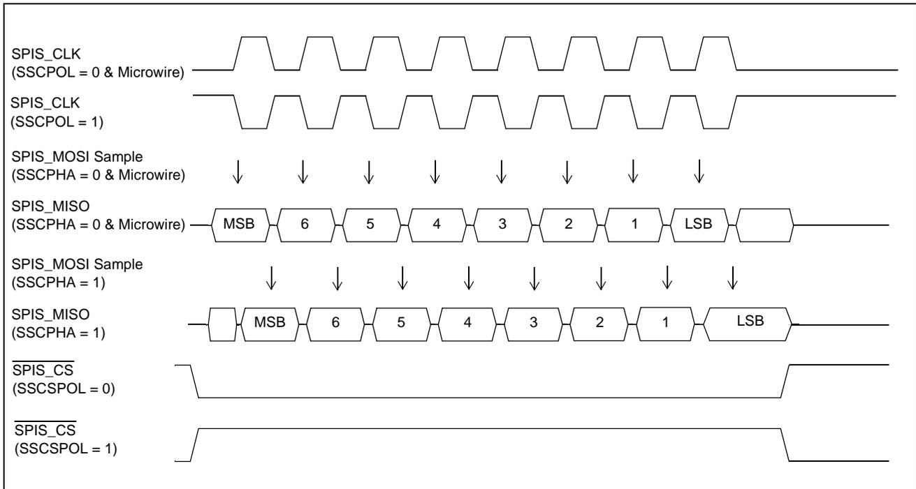
**Figure 23 - Slave SPI and Microwire Port Functional Timing**
