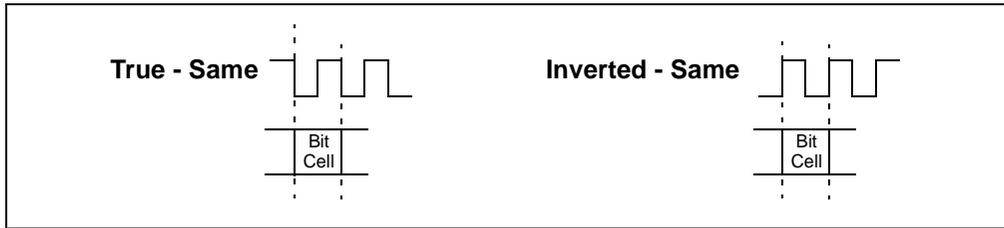
**Figure 7 - Clock Polarity versus Data Rate**
