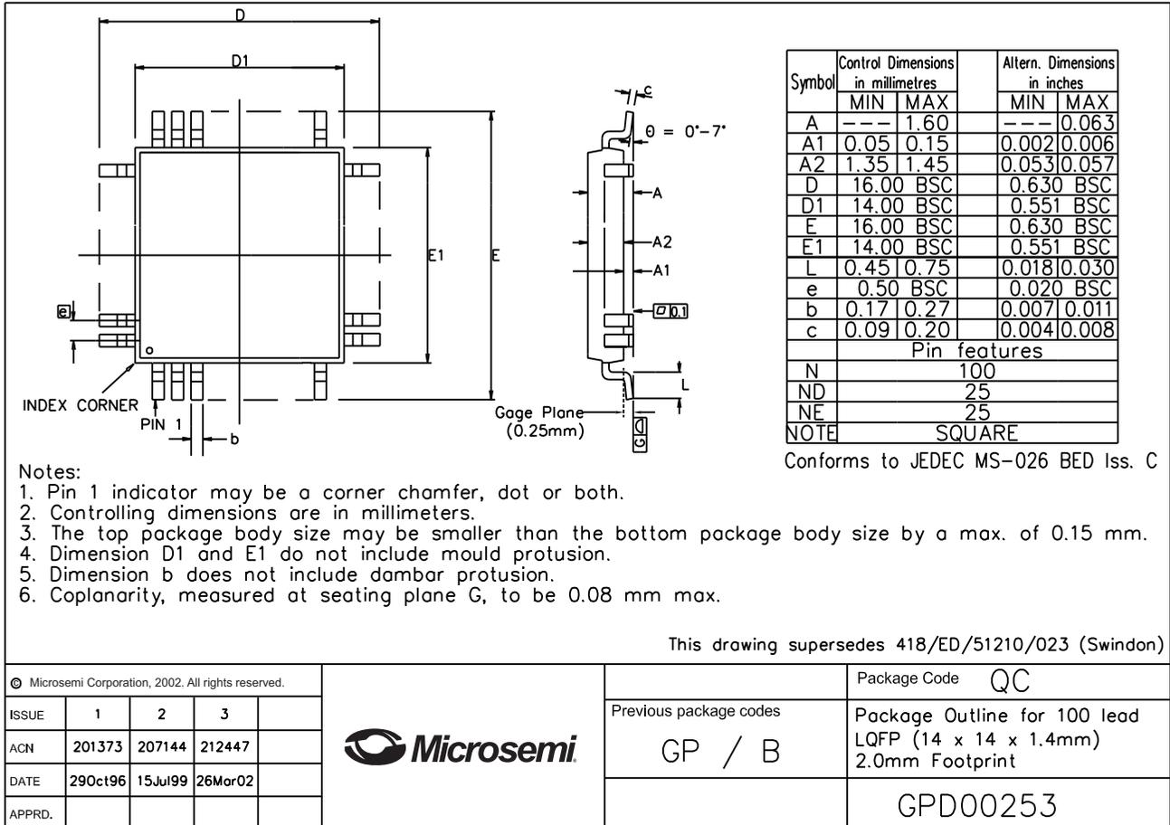
Figure 69 - ZL38004 (100-Pin LQFP) Package Drawing
