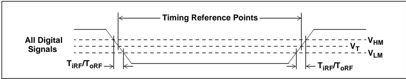
Figure 33 - Timing Parameter Measurement Digital Voltage Levels
