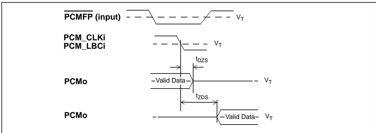
**Figure 41 - Output Tristate Timing in TDM Slave Mode**
