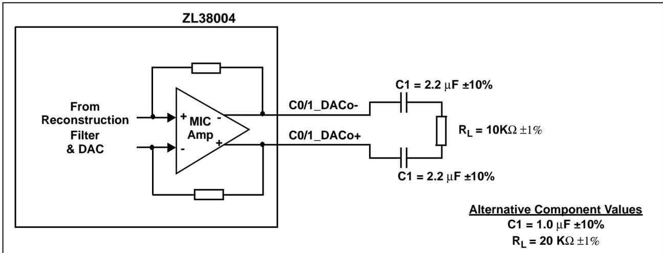
Figure 61 - CODEC 0/1 DAC Differential Driver Circuit
