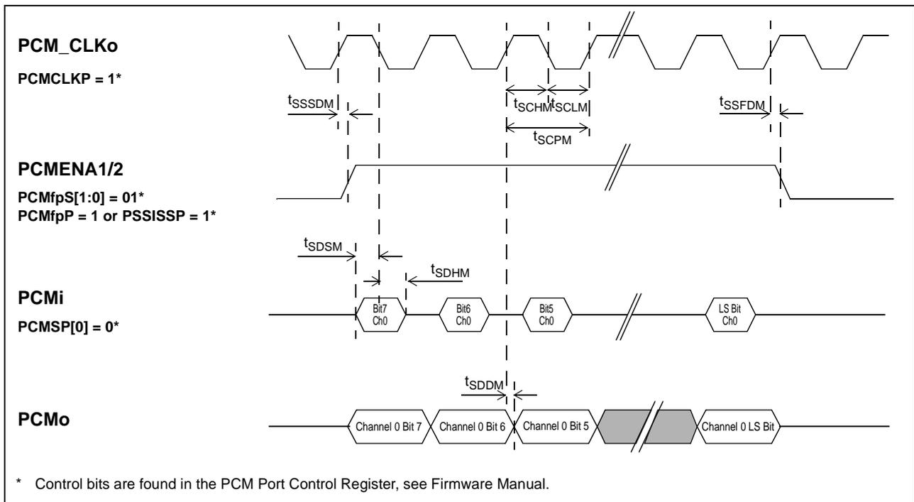
**Figure 35 - PCM SSI Master Mode Timing Diagram**
