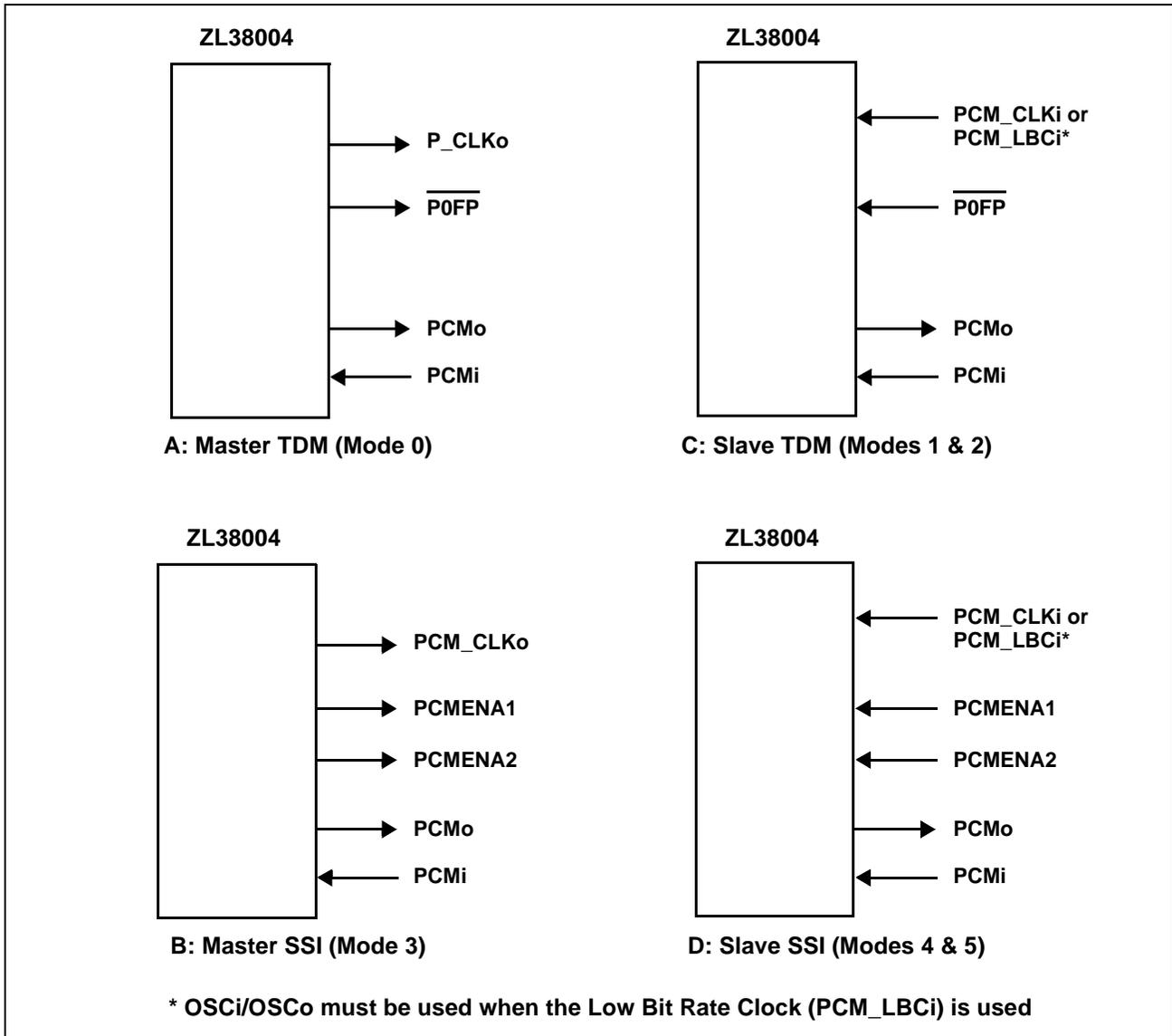
Figure 6 - PCM Port Signal Configurations for Master/Slave Operation
