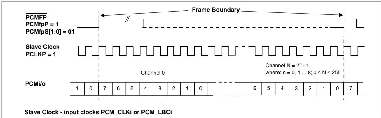
**Figure 11 - TDM - GCI Slave Functional Timing Diagram**
