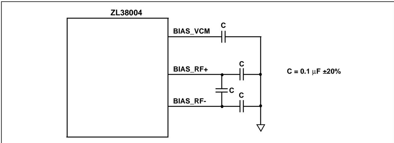
Figure 63 - CODEC 0/1 Bias Circuit
