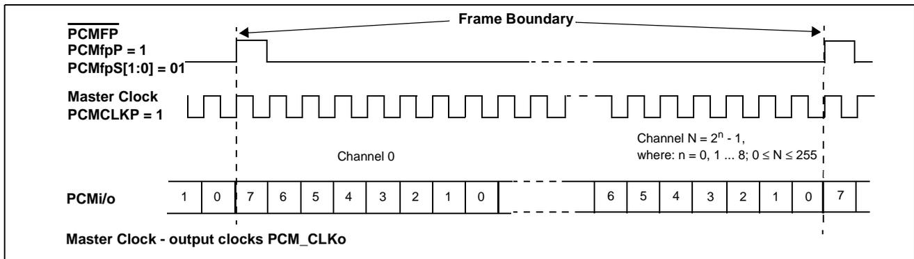
**Figure 12 - TDM - GCI Master Functional Timing Diagram**
