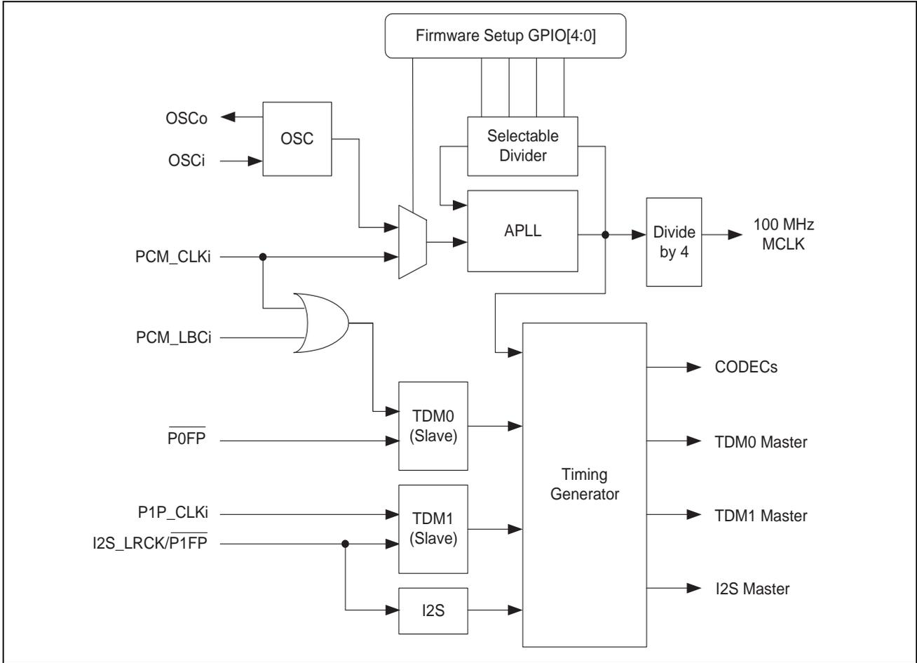
Figure 32 - ZL38004 Master/Slave Timing Selection and Clock Distribution
