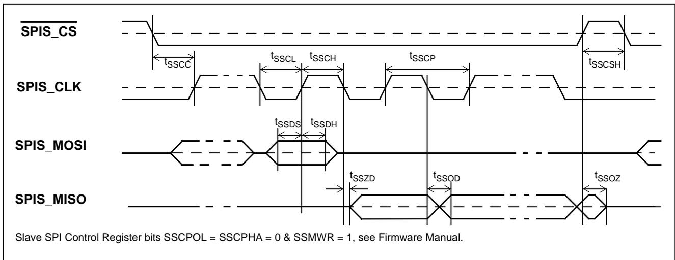
Figure 46 - Slave SPI Timing (Microwire mode)
