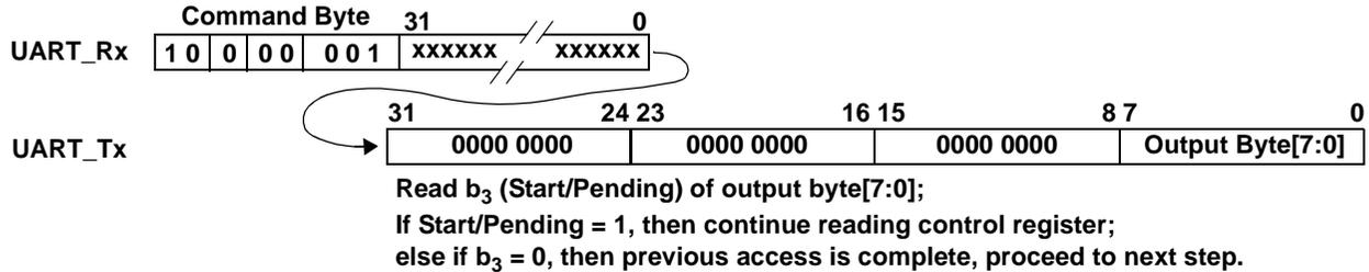
**Write 02A1<sub>H</sub> to Address Register**
