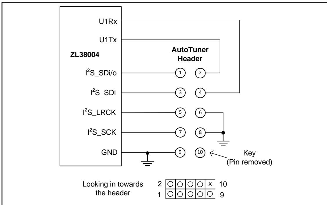
**Figure 68 - AutoTuner System Board Connection**
