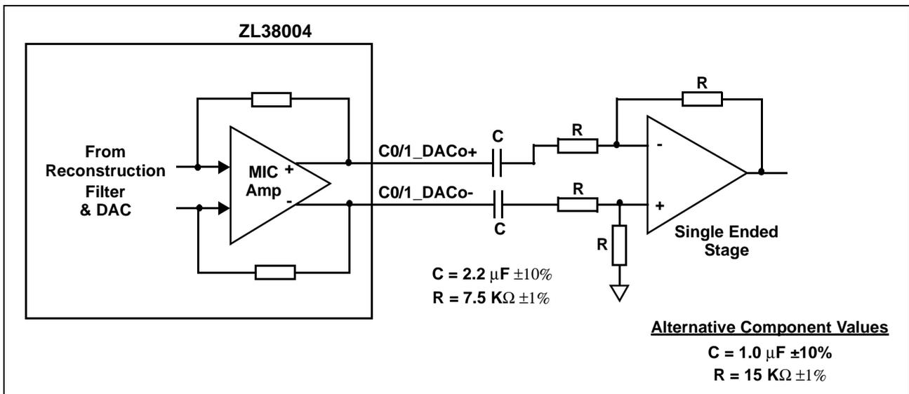
Figure 62 - CODEC 0/1 DAC Single Ended Driver Circuit
