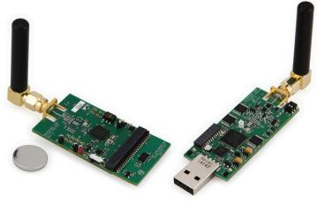
The included Z-Star protocol stack software supports Carrier Sense Multiple Access (CSMA) transactions in a star network configuration. This robust, proprietary protocol is optimized for ultra-low-power wireless sensor networks and minimizes both packet size and transaction time. The protocol stack may be further optimized for specific customer applications (for example, by varying packet length, latency, and frequency of transmission).
