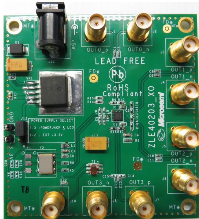
Figure 1: Top view of ZLE40203\_XO Evaluation Board
