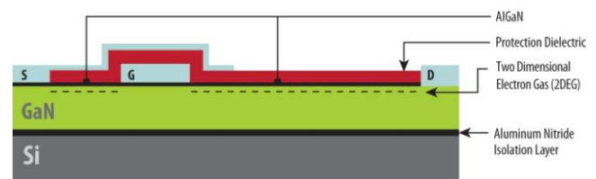
Figure 1. Simplified cross section of an eGaN FET
